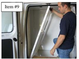
Position 3<sup>rd</sup> Compartment Bulkhead as shown above.
